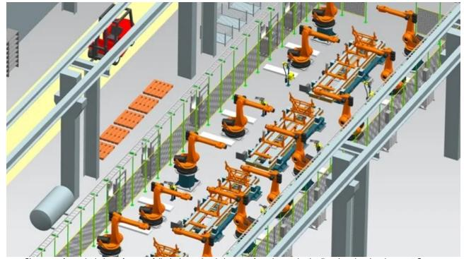
Siemens software includes software to fully design and optimise manufacturing production lines in a virtual environment. Source:
