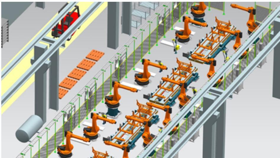
Siemens software includes software to fully design and optimise manufacturing production lines in a virtual environment.
